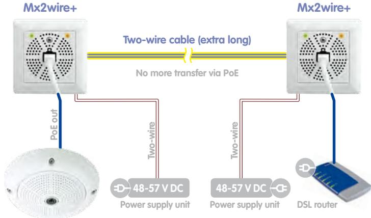
If the two-wire cable is not sufficient to supply the Mx2wire+ remote station with power due to its length, both Mx2wire+ units can be supplied with power via a power supply unit (48–57 V DC, 600 mA).
