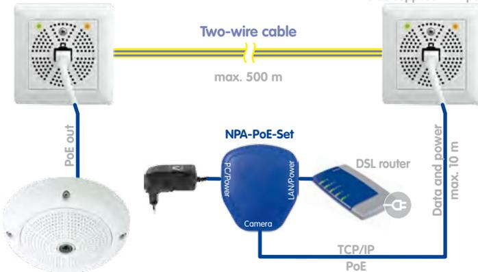
The NPA-PoE set (pictured here) or the weatherproof NPA box (not pictured here, available in 2012) are suited for standard PoE power supply according to IEEE 802.3af
