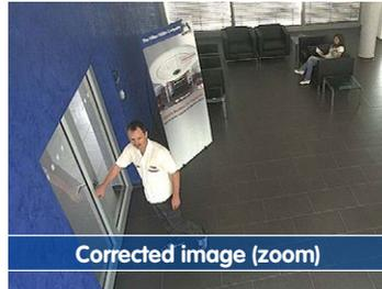
We recommend activating lens distortion correction, especially for applications with a low frame rate and non-zoomed images (for example, when using as a webcam). However, images can usually be corrected at a later point in time when searching recorded images. This saves on processing power during recording and increases the frame rate. The more you zoom in on the image, the less distorted the image should appear.
