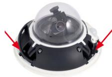
11. **Attach the outer shell:** Hold the outer shell so that the round hole of the shell is positioned over the PIR sensor of the camera. Gently press the shell into the shell's seats in the camera housing. **Old outer shells (D10D, D12D) may no longer be used!**
