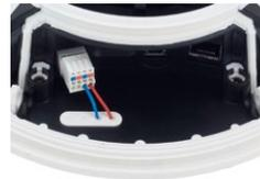
The white (detachable) MxBus connector has four connections (each of which is blue/red or +/-):
