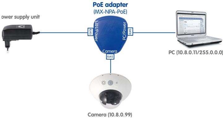
For the D15D you should use the blue MX-NPA-PoE-Set or the MX-NPA-Box - previous MOBOTIXnetwork power accessories, such as the NPA-Set, Power-Box and Power-Rack (MX-NPA-Set, MX-NPR-4 and MX-NPR8/20) are not suitable for use with the D15D.
