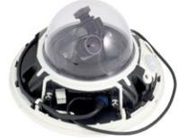
7. **Place the USB cable in the cable guides:** Carefully bend the cable guides upwards, place the USB cable in the guides and snap the cable guides closed again.
