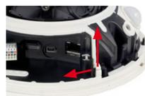
5. **Insert USB cable:** Insert the MOBOTIX USB cable from below through the cable outlet (see figure) and wrap it around the camera within the cable guides.
