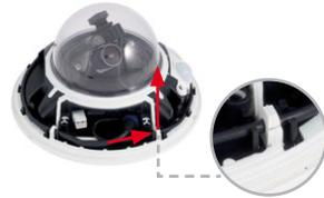
8. **Check the position of the cables:** The two cables should now cross one another just before the connectors.
