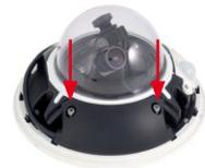
10. **Secure the cable:** Properly lead the cable through the cable guides at the outer rim of the housing and make sure that the outer shell can be properly mounted later on.
