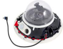
6. **Plug in the USB connector:** Insert the MiniUSB connector in the appropriate socket. Make sure that the cable is correctly fitted into the cable guides and that there is no excess cable in front of the connections.
