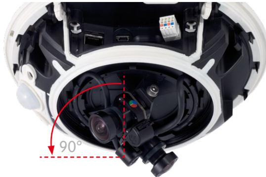
We do not recommend (even) aligning the telephoto lens horizontally due to the image distortions that occur in the top part of the dome for technical reasons.
