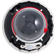
10. **Attach the outer shell:** Hold the outer shell so that the round hole of the shell is positioned over the PIR sensor of the camera. Gently press the shell into the shell's seats in the camera housing. **Old outer shells (D10D, D12D) may no longer be used!**
