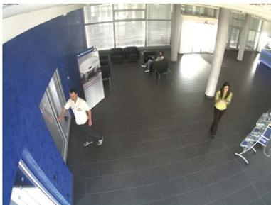
You can suppress this effect using software (for example, in the browser) so that a new and appropriately corrected image can be displayed live. A side effect of this correction, however, is that a cushion shape appears around the edges of the image.
