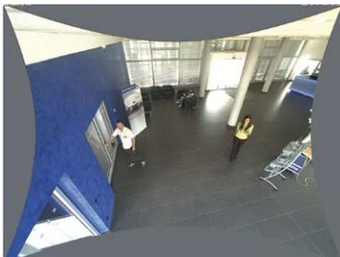
To hide this cushion effect, you simply have to **Zoom In** on the image slightly. Although this reduces the size of the captured area, the image is almost distortion-free compared to the original.
