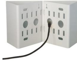
3. Insert the **supplied 10-mm screw anchors** into the screw anchor holes and secure the Corner and Pole Mount to the corner of the building using the **8x70 screws and washers (diam. 9 mm)**.
