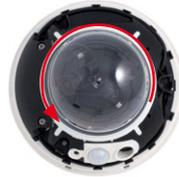
3. **Insert the lens units and mount the central lens screw:** Remove the center lock screw and the washer. Insert the lens units into the seatings. Insert the lock screw with a washer into the center of the camera and gently tighten it to hold the lens units in place.
