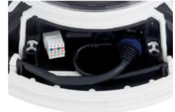
9. **Install cable cover:** Push the cable cover back into its seat and fasten the two M4x25 Allen screws. When mounting the cable cover, take care to properly align the cover with the seal of the camera housing and the two cable guides. This is the only way to ensure that the connections are reliably protected against any kind of weather.
