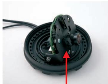
Insert USB plug into USB connector
