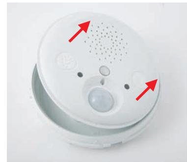
Remove the back of the housing
