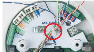
Lock the cable in place with cable tie and clip cable tie
