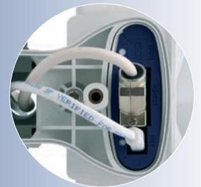
9) Guide the MOBOTIX M12 USB cable with the angled Mini USB plug first from below through the wall mount.
