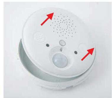
Remove the back of the housing
