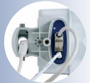
8) Reinstall the **bottom cover** of the mount. In the process, make sure that the camera's insect protection remains firmly in place.
